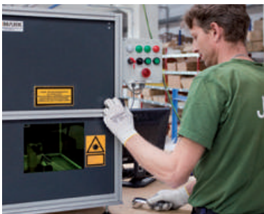
Laser beam during logo engraving process (II).
