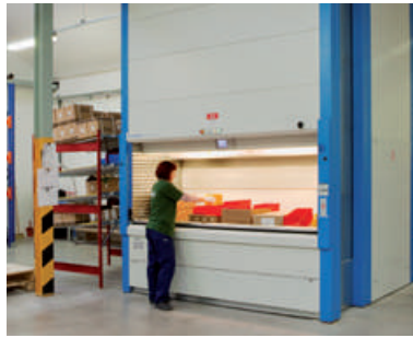
Kardex: automated high-capacity storage system.
